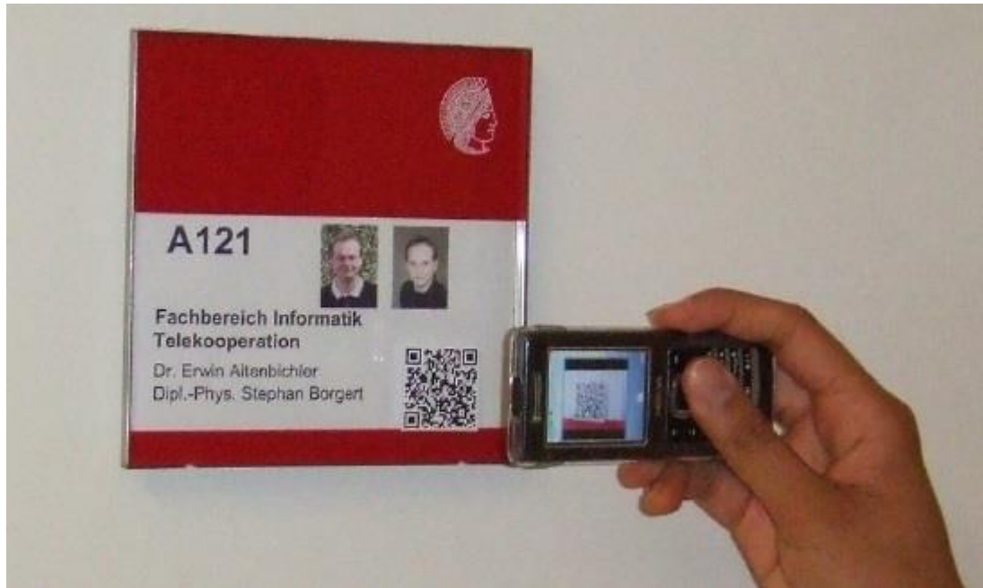
Figure 2: A QR code is scanned for use by IndoorNav, allowing it to find the user's current location. Such codes were distributed widely through the university building used in Russo's (2013) study.
